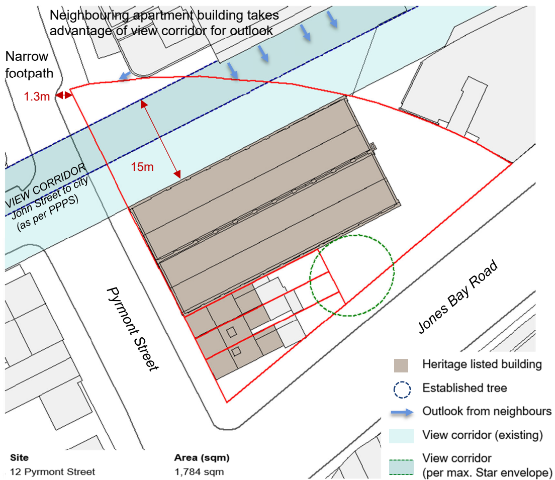
Figure 119 – existing site plan for 12 Pymont Street
